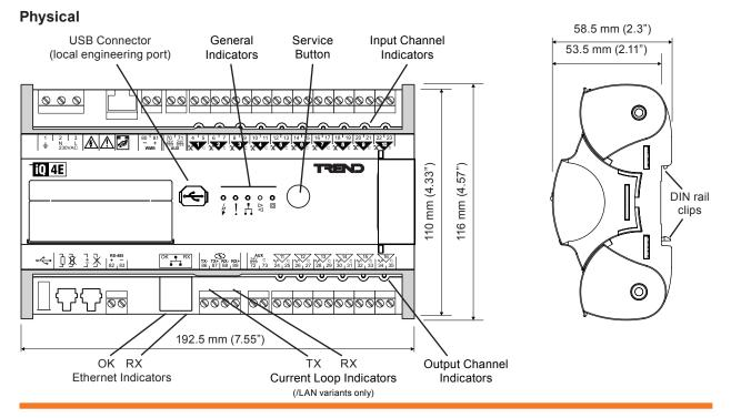
IQ4E/.. Controller Data Sheet TA201340 Issue 1, 28-Apr-2015. Applies to v3.30.
