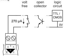
The volt free contact has a nominal wetting current of 270  $\mu A.$  The input is ON when the contact is closed.
